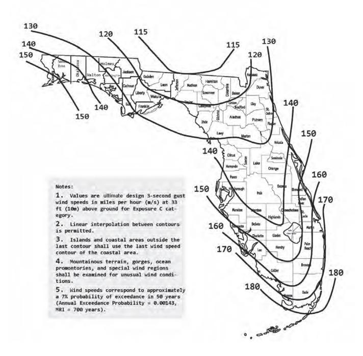
FIGURE 1609.3(1) ULTIMATE DESIGN WIND SPEEDS,  $V_{\scriptscriptstyle ULT}$ , FOR RISK CATEGORY II BUILDINGS AND OTHER STRUCTURES
